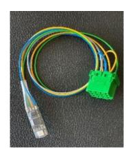
The emulator is mounted with the ignition switched off in the panel (wiring switchboard) under the hood in place of the original plug, which is the end of the wiring harness leading to the retarder controller - [8D] - photo on the left.
